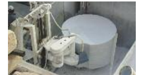
Cutter for carving column flutes.
