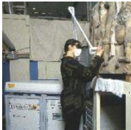
Cleaning of the west frieze in the laboratory using laser technique. (T.S.)
