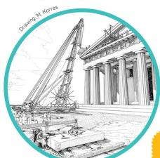
The lifting and positioning of the marble blocks was undertaken using various means: cranes, rope pulleys, rollers, and wooden or steel levers. The stability of the building was not secured using wet binding materials (mortars), as is done today. It was ensured through the perfect contact of the blocks, their proper positioning and the use of special connecting elements. Not even air could pass between the blocks.
