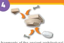
The fragments of the ancient architectural members and the new supplements are joined together using titanium rods, which are inserted into surfaces hidden from view.
